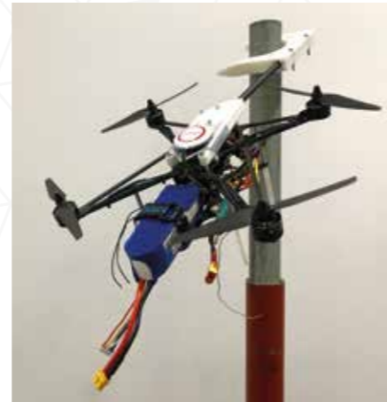
Figure 3 - Perching clamp tested on mockup metal column.
