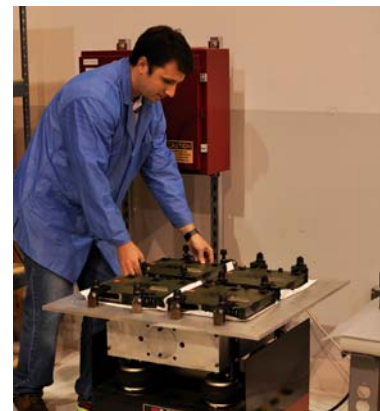
Vibration testing identifies defects prior to shipment.
