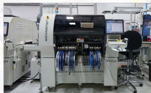
7-Spindle High Speed SMT (16,500 CPH Placement)
