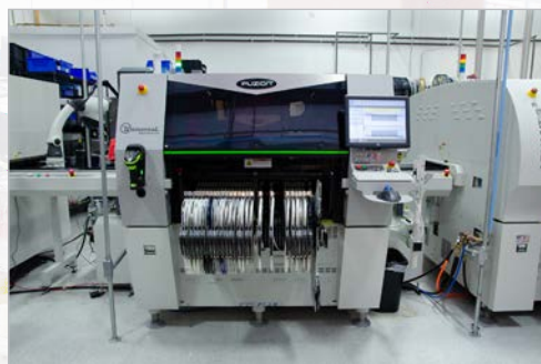
60-Spindle High Speed SMT (60,000 CPH Placement)
