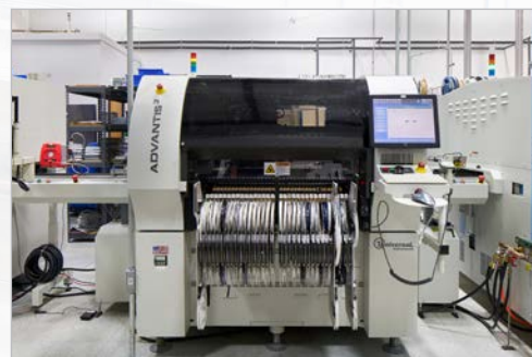
30-Spindle High Speed SMT (34,500 CPH Placement)
