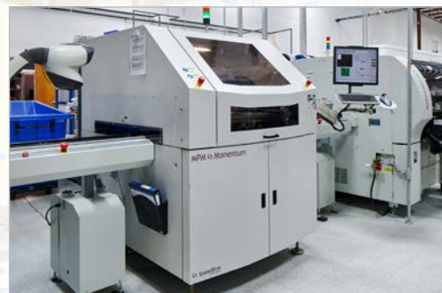
Automated Screen Printer with 2D Inspection
