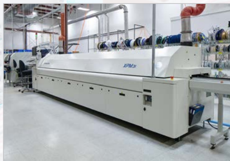
Ten Zone Forced Convection Reflow Oven
