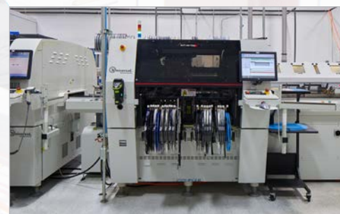
7-Spindle High Speed SMT (16,500 CPH Placement)
