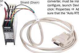
Note: RTS is only required to be connected if using software controlled RS-485. The SeaCOM driver, which is included with the converter, must be installed and configured for (RTS) RS-485. To configure, launch Device Manager, select Com [XX] Port ⇒ right click: Properties ⇒ Advanced tab. On the Advanced tab, make sure that the "Auto RTS RS-485" check box is selected.
