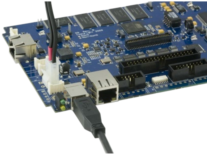
Figure 3 – Connect the Type B connector to the SBC-R9
