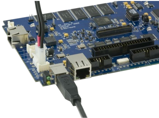
Figure 42- TR123 tinned leads and Type B USB connector
