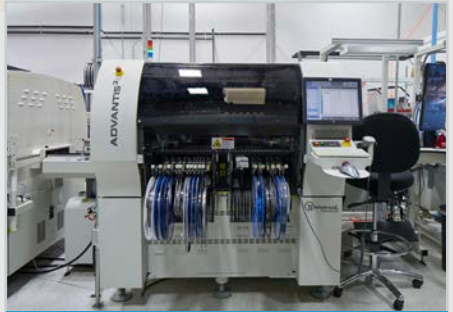
7-Spindle-High Speed SMT (16,500 CPH Placement)
