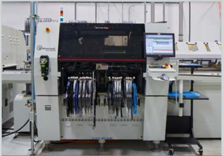
7-Spindle-High Speed SMT (16,500 CPH Placement)
