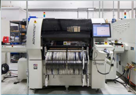
30-Spindle-High Speed SMT (34,500 CPH Placement)
