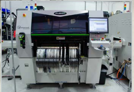
60-Spindle High Speed SMT (60,000 CPH Placement)
