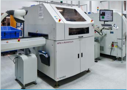
Automated Screen Printer with 2D Inspection
