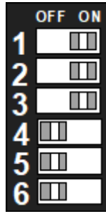
Figure 6 – RS-422 with Termination and Receiver Echo
