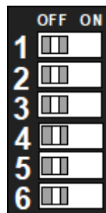
Figure 5 – Dip switch SW2, Line Termination and Echo Off/On
